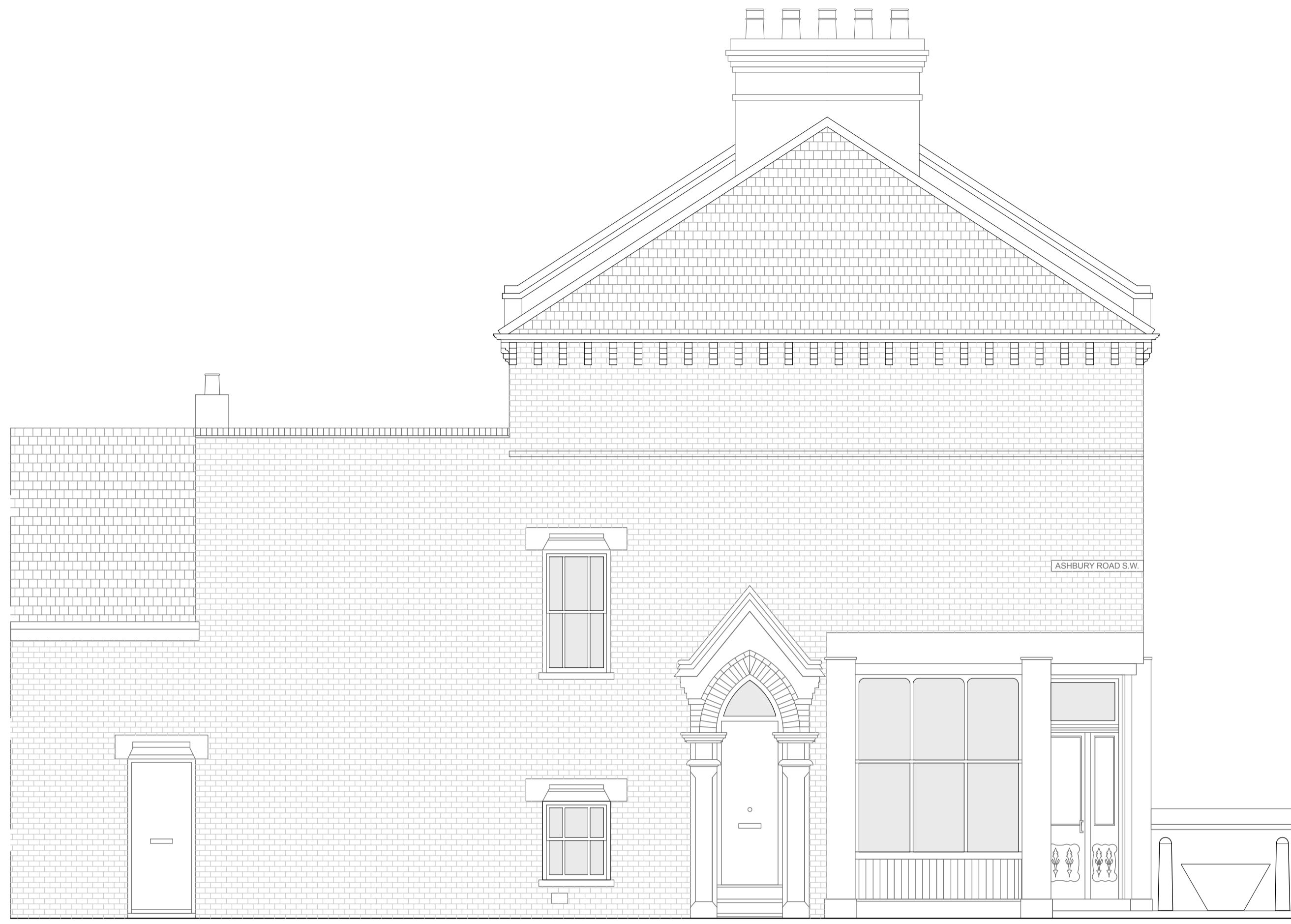
1 NORTH ELEVATION AS EXISTING SCALE 1:50
